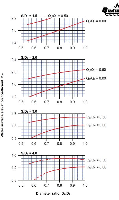
Water surface elevation coefficients (K<sub>w</sub>) for 22.5° bends at pit junctions with branch point located on the upstream face of pit for submergence ratios  $S/D_0 = 1.5, 2.0, 3.0$  and 4.0 (Source: Hare, 1980)
