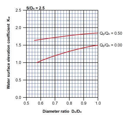
Water surface elevation coefficients (K<sub>w</sub>) for 22.5° bends at pit junctions with branch point located on the upstream face of pit for a submergence ratio  $S/D_0 = 2.5$  (Source: Hare, 1980)
