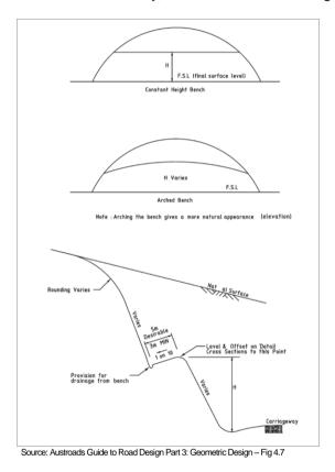
Figure D1.10 - Elevation and cross section of benches
