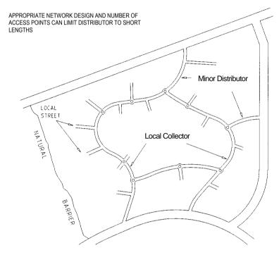
Figure D1.5 - Local Collector and Minor Distributor
