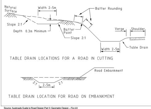
Figure D1.11 - Typical table drain shape and location
