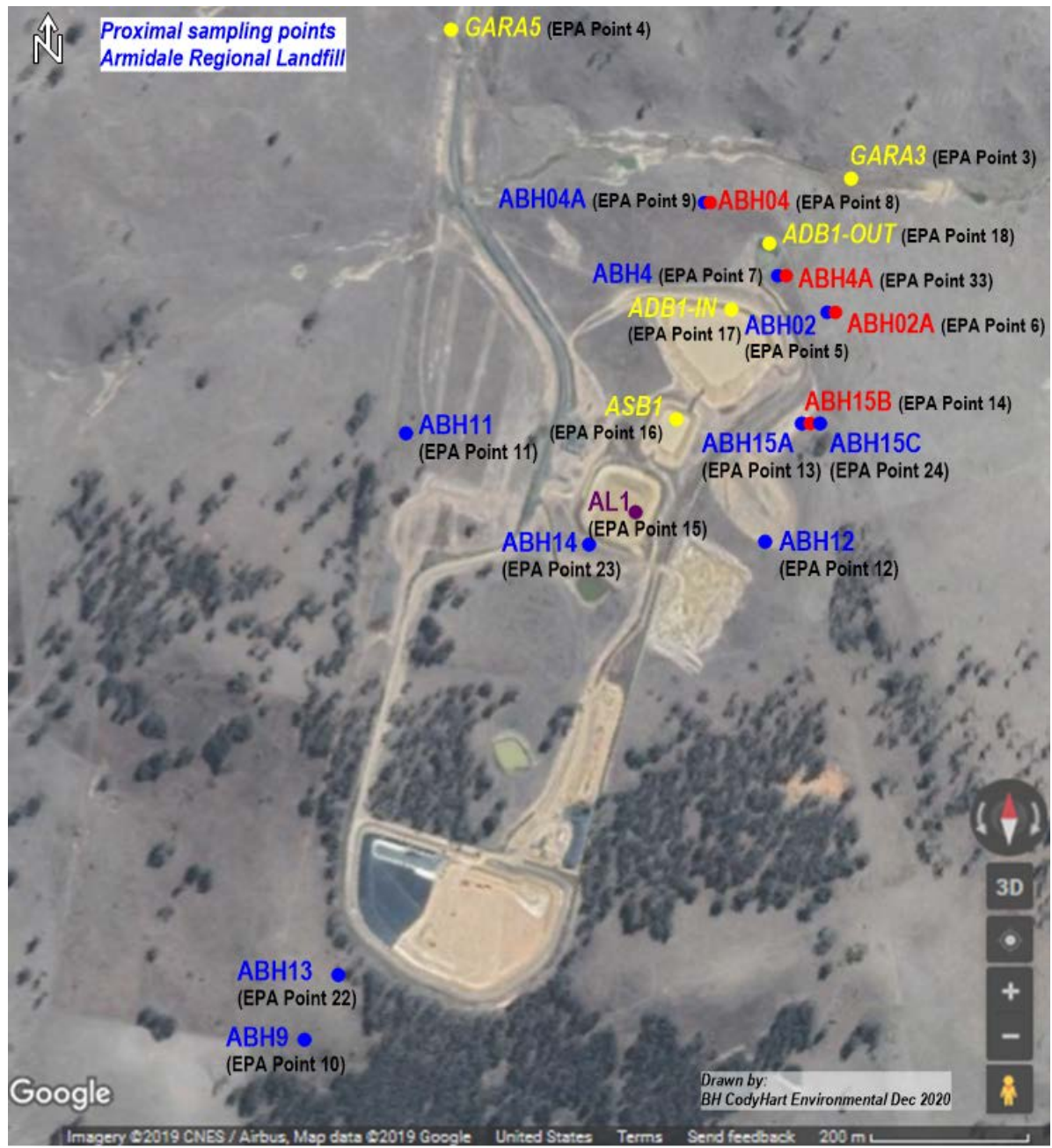
Figure 1: Proximal groundwater and surface water sampling points, Armidale Regional Landfill
