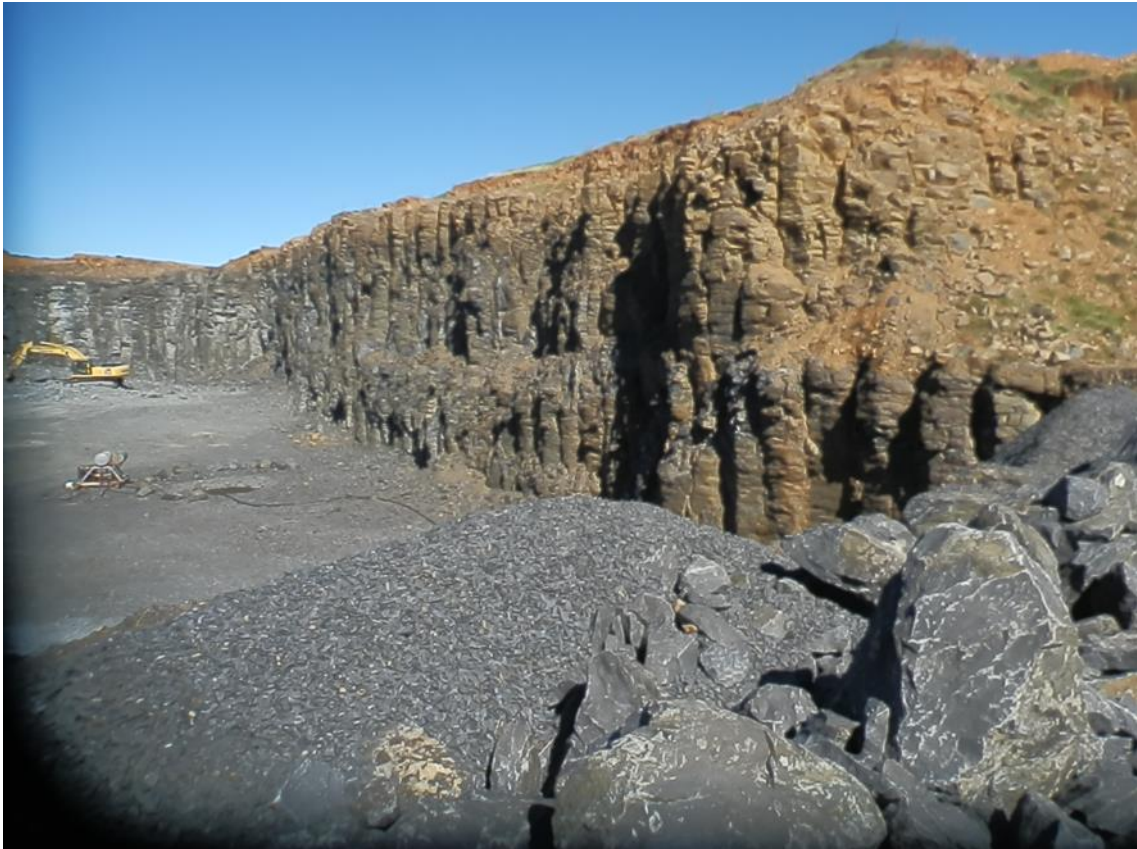
Plate 30: General view of the quarry face (Site 4) showing shallow residual, bouldery profile overlying more competent basalt.
