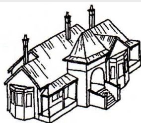
Grander Federation homes adopted much more complex forms, particularly in roof shapes. Corner sites were especially favoured.
