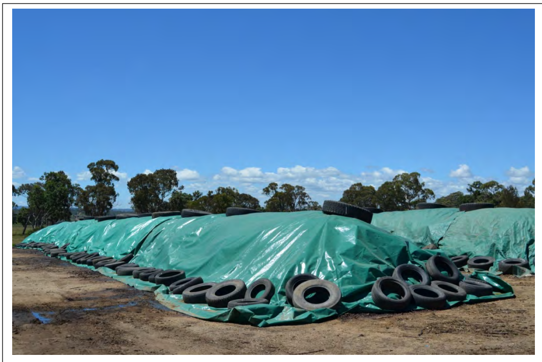
Photo 14. Food organics green organics in windrows, note that the tyres are used to hold the tarpaulins which are used repeatedly down and prevent them from blowing in the wind.
