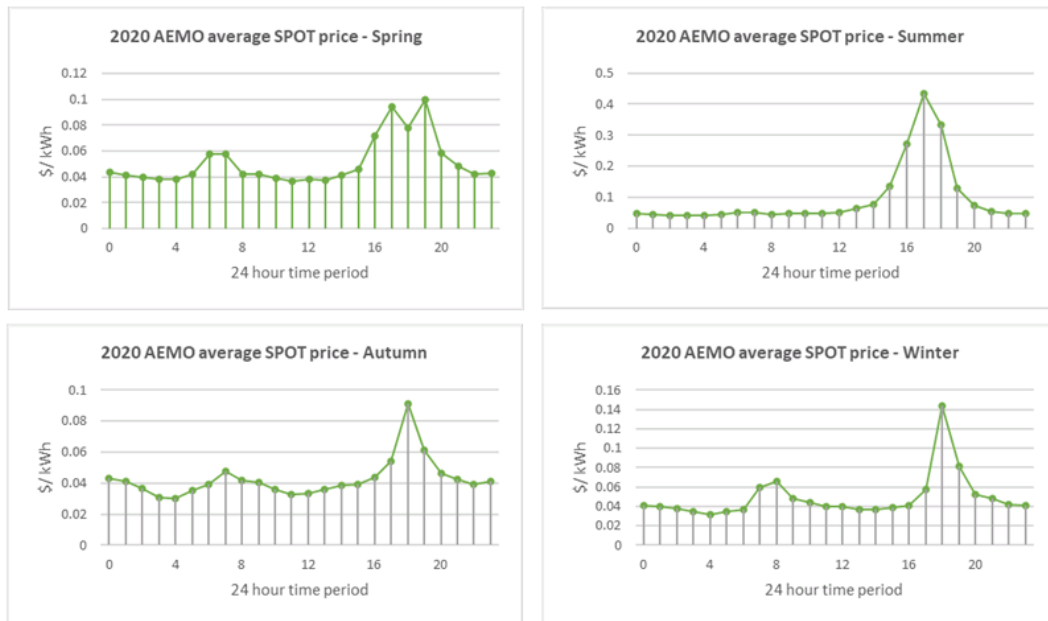
Chart 6. Seasonal average AEMO (Australian Energy Market Operator) NEM Spot electricity price charts
