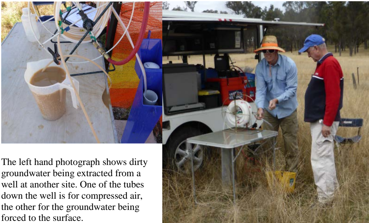
Photograph 1: Well development by pump out
