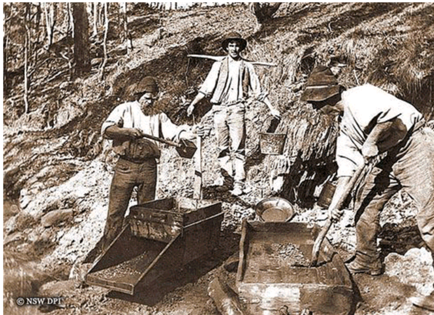
Photograph 4: Cradling for gold at Box Ridge, near Sofala, NSW. Circa 1870.
