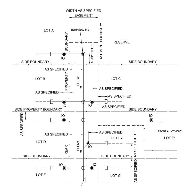
TYPICAL CONNECTION METHODS FOR SEWERS IN EASEMENTS (REAR OR SIDE BOUNDARIES)
