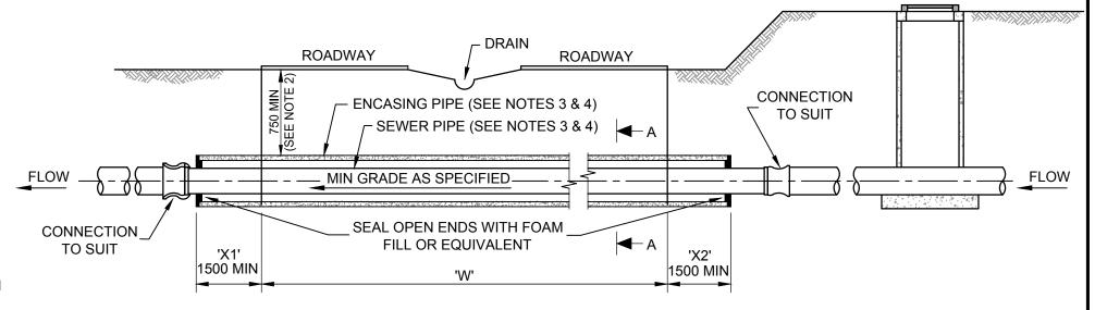
BORED OR JACKED ENCASING PIPE METHOD
