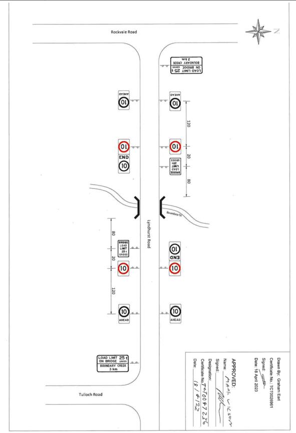
Plan - TGS for Load Limits on Bridges
